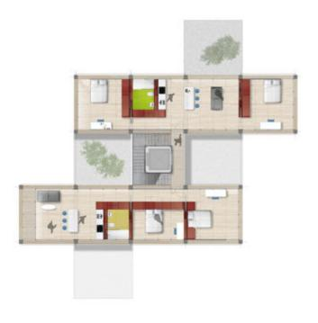
The units are stacked, using a simple gravity structure, around a central stair and lift. Minimal foundations are required.
